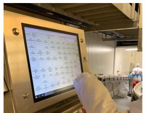
At Bahlmann, the product feed is visually checked by the employee on the conveyor belt and selected directly via the machine terminal. A visual product segmentation via a camera system is also possible. The product information stored in a database is then forwarded to the labeling system and label printing starts in real time. All this with small product batches up to batch size 1 and speeds of up to 100 packs per minute.
