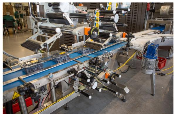
After the double check on the scale the label with weight indication subsequently follows. When it comes to the harder type of fruit or vegetables, the machine can press more firmly. But if there are grapes on the line, then the machine stamps with special care.
